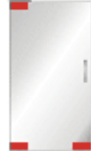
Single Door with Patch Fittings, Closer, Lock
